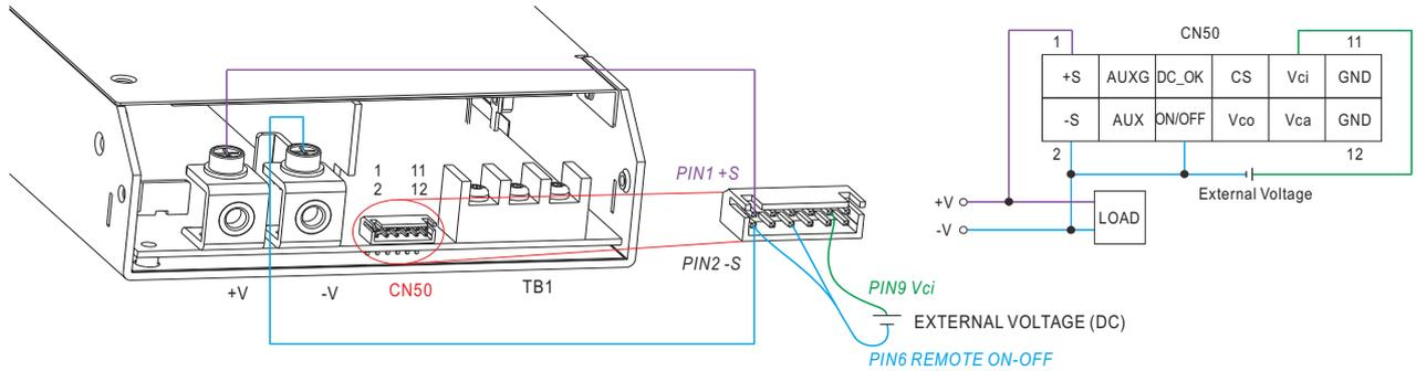
◎ +S & +V and -S & -V also need to be connected on CN50
